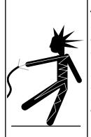
This equipment must be grounded. Verify that any existing electrical outlet and circuit you intend to plug into is actually grounded. Under no circumstances should the grounding pin from any three-pronged plug be removed. Serious injury may occur.
